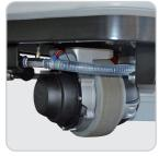
TRACTION MOTOR WHEEL: permits a great maneuverability. The machine rotates completely in 210 cm wide corridors!
